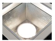
DARK LIGHT (PLASTIC REFLECTOR), SQUARE LED Reflector is made from one piece injection moulded Polycarb with full specular 99.98% Reflectance Value Vacuum Metallised finish. The design minimizes glare to maximize visual comfort together with maximum light
